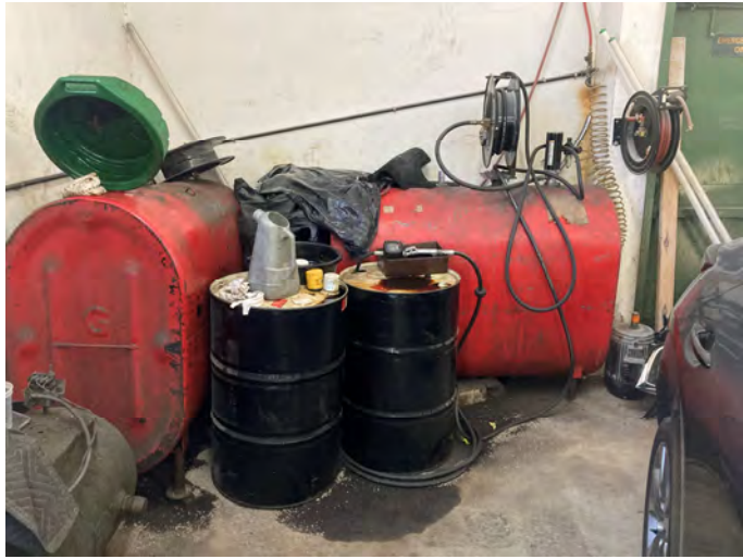
05 Two 55 gallon drums and two ASTs used for motor oil inside the 435 Wales Avenue garage with staining present on the concrete floor.
