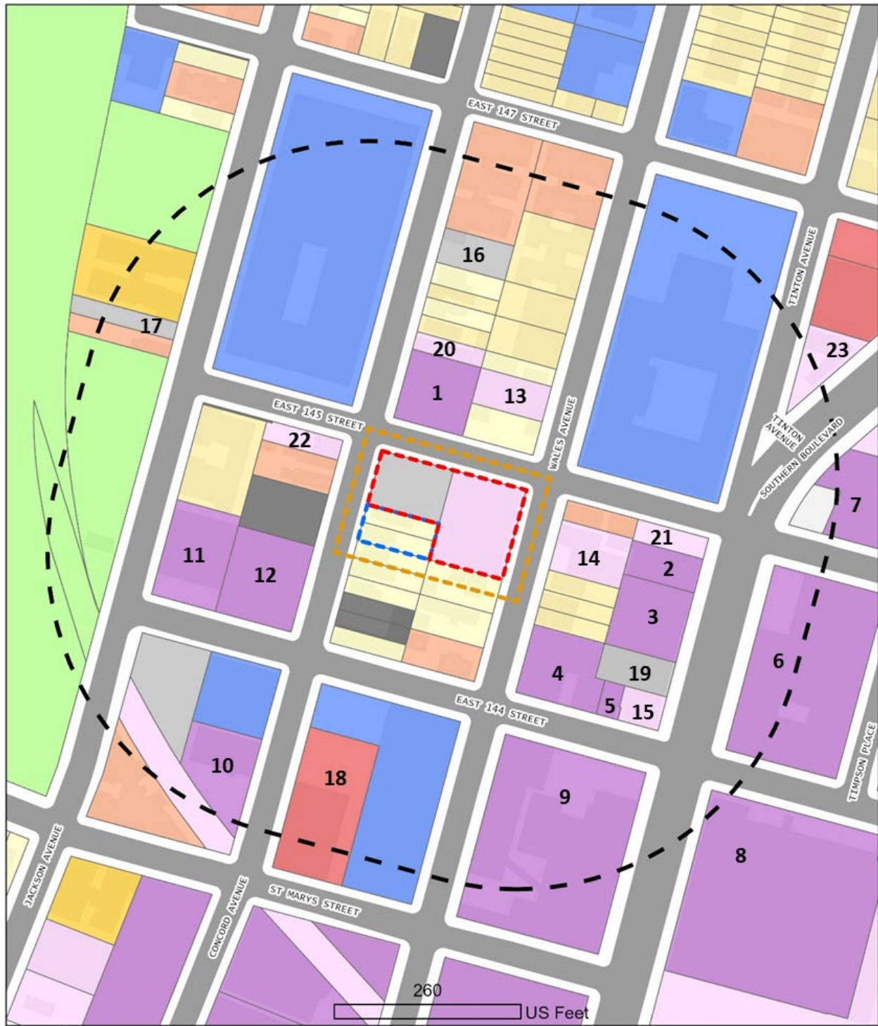
Figure 2.8-3: 400-Foot Industrial Emissions Screening
