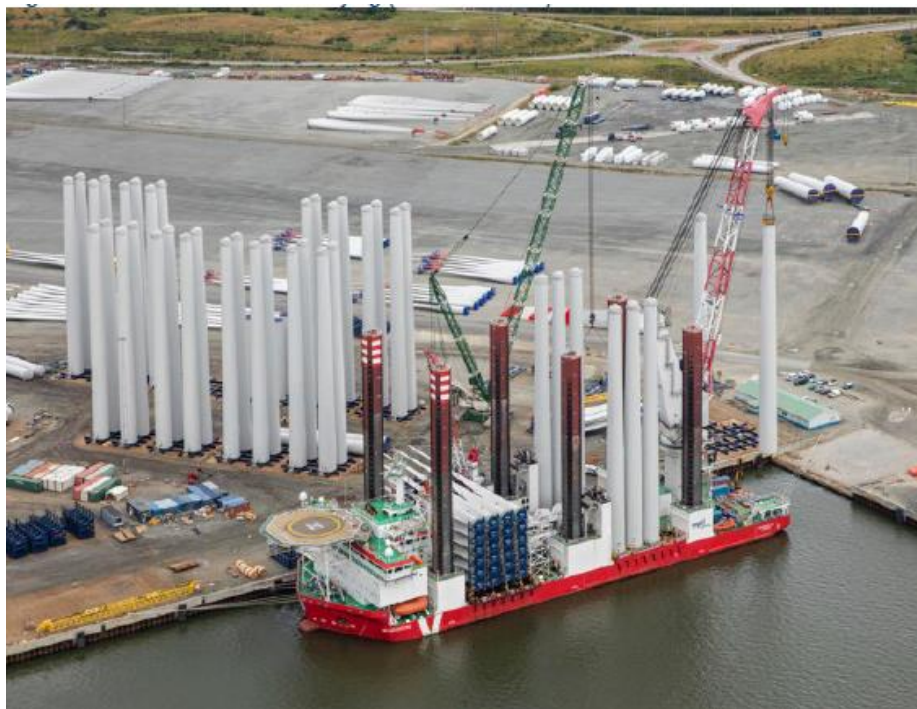
Figure 2: Wind turbine components loading activities to WTIV
